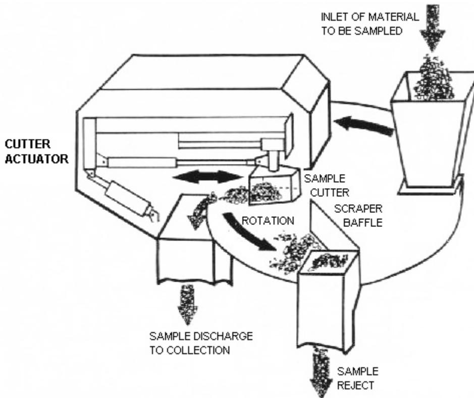
The ROTARY TABLE SAMPLER enables efficient sampling of powders and solid materials including moist concentrates and other material having tendencies toward sticking to chute surfaces when using trajectory or top-belt sampling. The rotary table method also is efficient for sampling fine powders by avoiding sample bias resulting from fines classification occurring with gravity flow sampling. It is used for secondary or tertiary sampling, or for primary sampling of relatively small flows.
