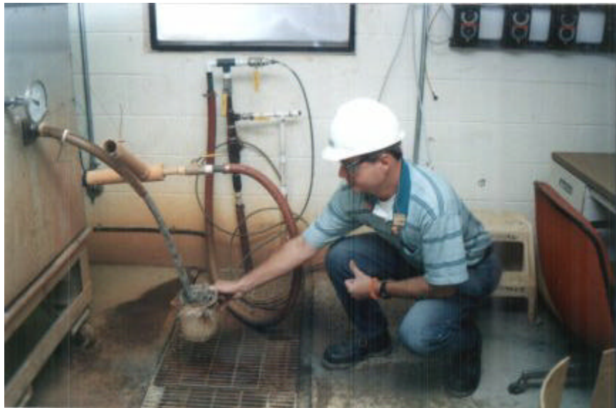
FIGURE 7. Test Sample Collection during Slurry Flow through the Phospholyzer™
