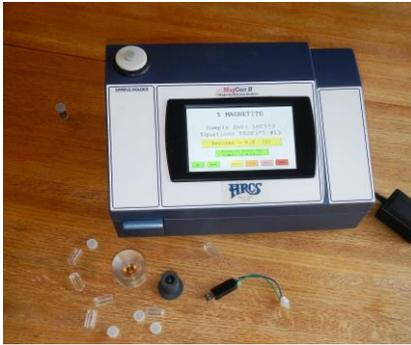
**Analyzer Use:** The **MagCorrII** has a user-friendly operating menu with selections for compaction, analysis, calibration, trends, and data collection / storage. The analyses data and the calibrations used to calculate those data are available for user computer access.
