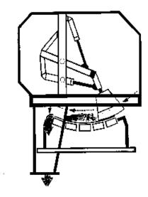
The PRX Top-Belt rotary cutter sampler is designed to extract representative samples directly from solid materials carried on a moving conveyor belt. Extraction takes place by driving the PRX cutter through a circular path above the belt with radius of the path matched to arc radius of specially constructed supporting belt idlers installed on each side of the cutter. The supporting idlers establish a fixed belt contour at the sampling position.
