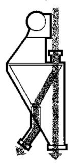
The PRV rotating sampler is designed to be installed with gravity flow streams of relatively fine, non-adhering solids material to obtain representative composite sample. Chute angles are maintained at 60 degrees or greater for effective discharge and minimize build-up on interior surfaces. The mechanism is designed for rugged, heavy-duty use and for low maintenance in continuous service.
